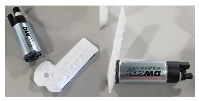
20 – Slot the pump into the filter assembly. It will only clock in one way. Now take the filter assembly with the pump and slide it into the bucket. It will only go into the bucket one way. The venturi hose on the top left of the 2<sup>nd</sup> picture is an easy marker if the filter is being installed correctly as there is a groove for the hose.
