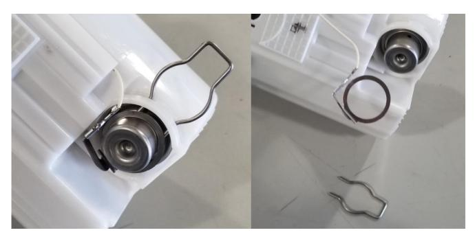
6 – There is another small static ground on top of the filter assembly. To remove it, depress the small tab and pull on the wire.
