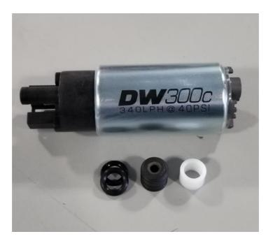
18 – Below is a picture of the OE seal and the new o-rings. Either method can be used.
