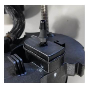
14 – We need to replace the venturi hose. Use a razor blade to cut the hose shown in the 2<sup>nd</sup> picture. Take care to not damage the barbs under the hose.
