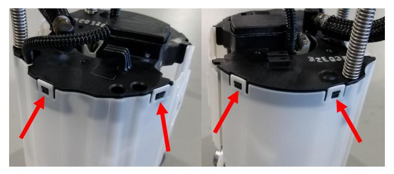
10 – Once the filter assembly is removed, on the bottom side of it lies the pump pre-filter/retainer. Unlatch the tabs and pull the pump out of the filter assembly.
