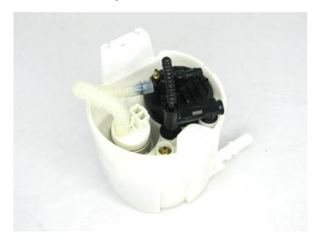
2 – remove the venturi manifold by prying up from the middle with a screwdriver or lever
