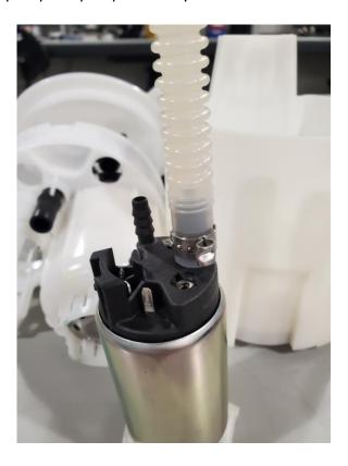
6 – Attach the supplied 1/8" venturi hose to the venturi jet inlet on the bucket and clamp with the 6.1mm clamp. Install the center section into the bucket. Make sure to snap the venturi jet assembly back into place.
