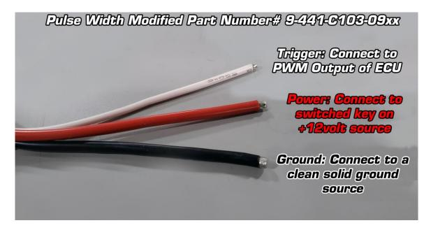
12c – If your ECU outputs a pulsed positive signal it will have to be converted to a ground signal before you can use the Deatschwerks Brushless Controller. Follow the wiring diagram below to install the signal adapter.
