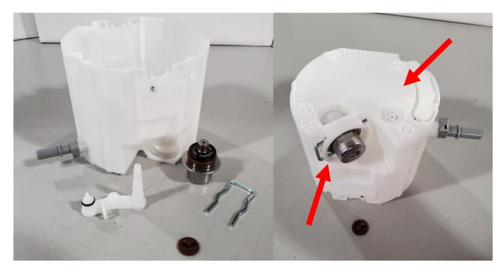
6 – Install the rubber one way valve into the bottom of the bucket.
