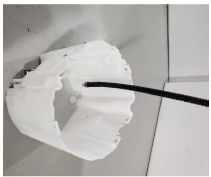
8 – Install the completed hat and pump assembly into the bucket assembly, there is a hole in the orange center section directly above for the venturi hose to pass through.
