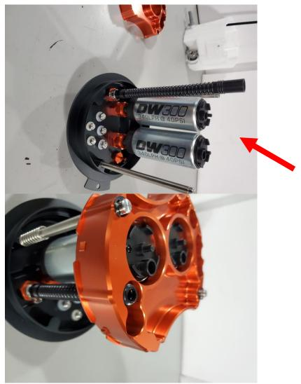
3 – Install the two supplied fuel filter socks onto the bottoms of the pumps, be sure to remove the clear plug from the filter sock, and the red cap from the fuel pump.
