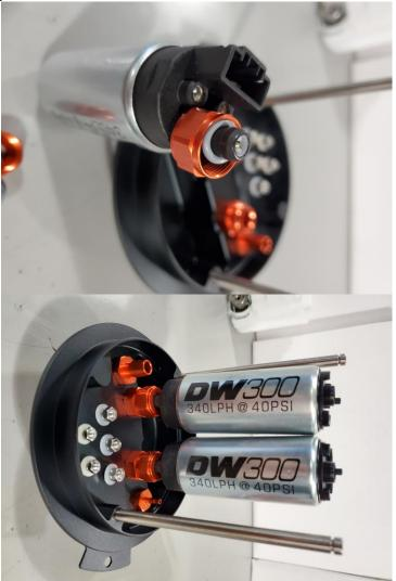
2 – Install the supplied 3/8" convoluted tube onto the return fitting and secure with the supplied 3/8" pinch clamp. Slide the center plate over the pumps and return tube, reinstall the e-clips, cut the return hose flush with the bottom of the return plate when its fully extended.
