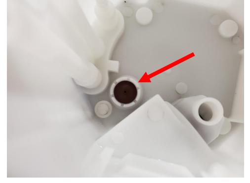
7 – Install the supplied smaller convoluted hose onto the venturi jet nipple inside the bucket, secure with the 8.5mm hose clamp.
