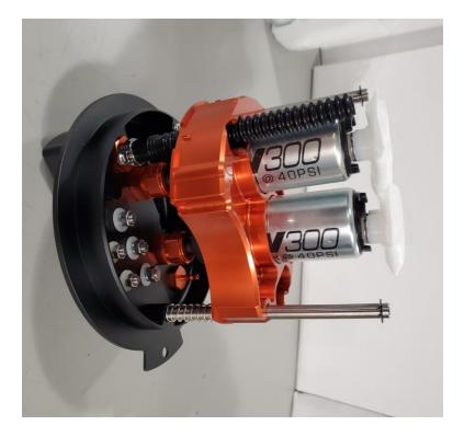
4 – Shorten the supplied wiring harness to approx. 8-inch (205mm) and crimp on the supplied ring terminals. Attach both ground wires to the pump negative terminal and attach each pump power wire to its separate positive terminal. Tuck the remaining wire into the cavity provided above the pumps.
