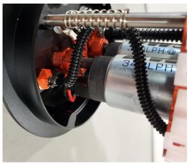
10 – Strip the ends of the provided fuel level sending unit wiring and crimp on the provided ring terminals, it may be necessary to double the wire over due to its small size. Attach the level sending unit wiring to the Level positive and negative terminals.
