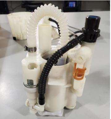
8 – Install the pump and filter assembly back into the bucket, make sure all locking tabs are in place and secure.
