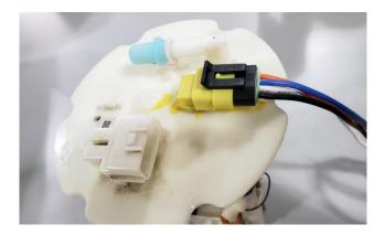
12 – Plug the 3-wire pigtail harness into the controller.
