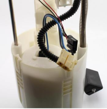
2 - disconnect the venturi jet and separate the fuel level sender from the assembly
