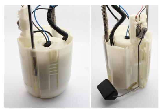
8 – reinstall the assembly into the fuel tank and attach a length of hose to the outlet of the pump assembly allowing it to drain into a fuel safe container and prime the fuel pump assembly
