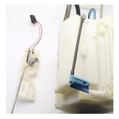
3 – separate the bottom from the assembly by opening the 3 tabs (green circle) and removing the retainer clip from the upright
