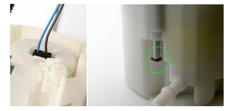
4 – unclip the fuel sock form the center assembly and pull the fuel pump out
