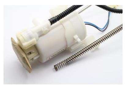
7 - install center assembly into bucket and reconnect the fuel level sender
