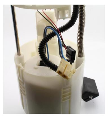
2 - disconnect the venturi jet and separate the fuel level sender from the assembly
