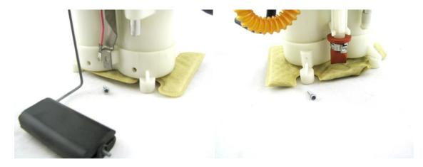
2 – pry the fuel sock off the pumps and then pull the base away from the assembly
