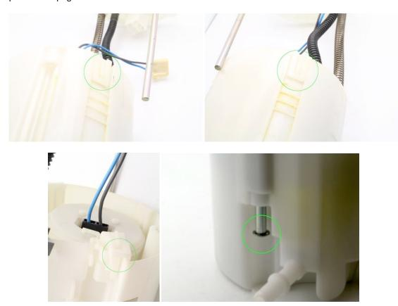
4 – unclip the fuel sock form the center assembly and pull the fuel pump out
