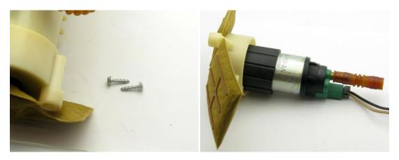
3 – remove these parts from the OE pump, they will be reused for installing the DW300m, the sock supplied in the DW installation kit is for use if the OE sock is not serviceable
