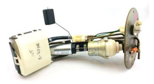
8 – reinstall the assembly into the fuel tank and attach a length of hose to the outlet of the pump assembly allowing it to drain into a fuel safe container and prime the fuel pump assembly
