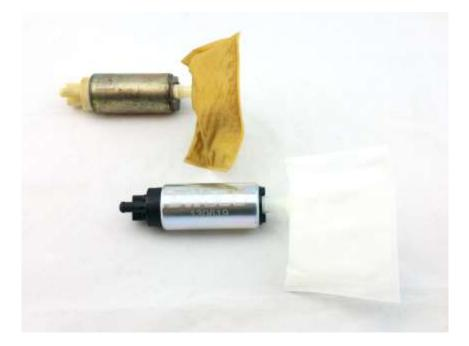
4 – measure and cut the supplied hose, then install it onto the assembly inlet. Slide the new hose clamps on the hose toward the top of the assembly and install the DW200/300 with the supplied isolator on the bottom of the pump. The supplied electrical connector is for earlier Impreza models that came with a different pump connector design. The OE connector can be retained
