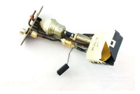
1 - remove the fuel sock cover from the base of the assembly
