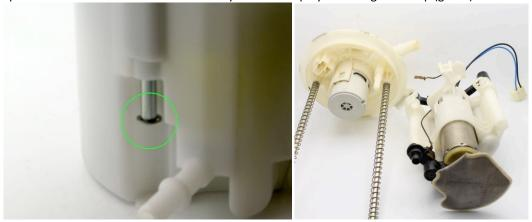
4 – remove the fuel pump from the center section by using 2 flat-head screwdrivers to open the retaining tabs (green)
