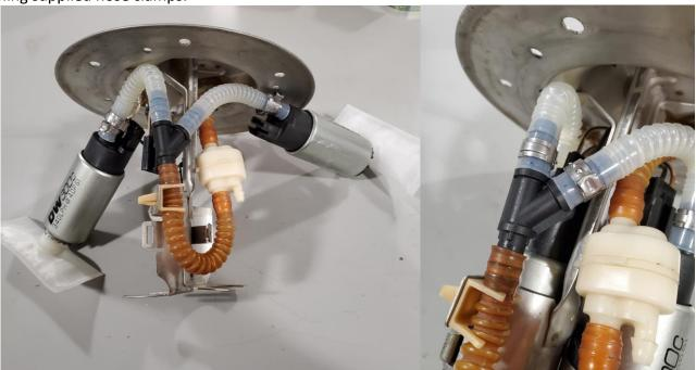
8 – Plug the factory connectors back into the pumps, due to the special notch that's been added to the Deatschwerks pumps the factory connectors plug directly into the new pumps. Re-install the factory band strap onto to the module, hook the end through the eyelet on the module and secure with the OEM 9/32" screw.
