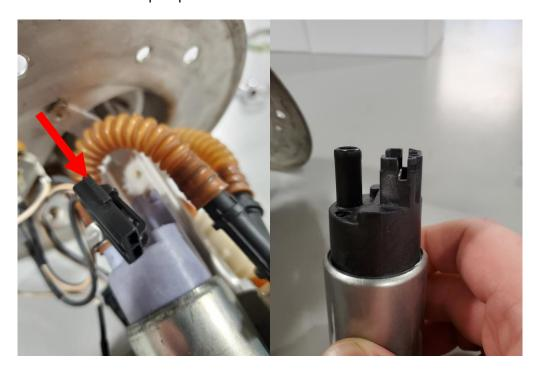
4 – Remove the factory convoluted tubes from the top of the Y-Fitting. This is typically done with a knife, take care not to damage the fitting under the tubing. Once loose remove the pumps from the module.
