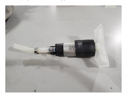
6 – The supplied convoluted fuel hose has different sized openings at each end. The smaller end is designed for the Deatschwerks fuel pump, slip it on and secure it with one of the supplied hose clamps, repeat this on both fuel pumps.
