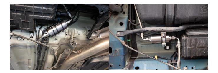
6 – Continue running the rest of the AN hose up into the engine bay. Locate a suitable mount for the adjustable fuel pressure regulator, here it is bolted to an available bracket on the engine, and the firewall. The 6AN hose will now be the new feed line, it should connect to the side of the regulator.
