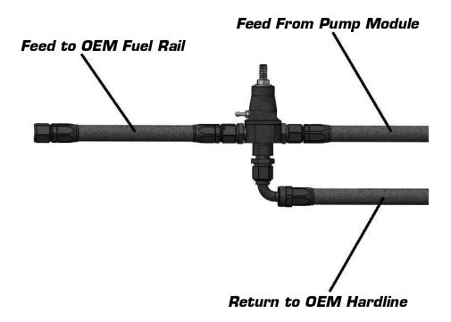
8 – Remove the factory plastic/rubber fuel line that connects the hardline on the firewall to the factory fuel rail. Use the included 1/4" Female EFI Quick Connect to 6AN adapter to adapt the hardline on the firewall into the new return line. Plumb this fitting into the bottom of the provided DWR1000 regulator.
