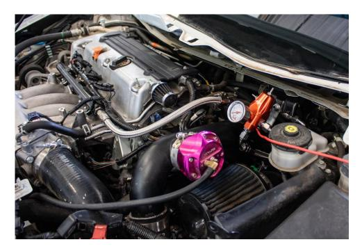
10 – Install any remaining hose ends with the appropriate angles needed for fitment, plumb the regulator, fuel filter and fuel rail as shown in the diagram in step 7. The last step is to attach the fittings to the module. Reconnect the factory plastic hose to the factory quick connect fitting on the top hat of the DW400 module. Attach the new 6AN feed hose to the 6AN bulkhead fitting. Re-connect the vent hose and the electrical connector.
