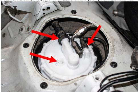
2 – Using the appropriate tool, remove the lock ring that holds the pump into the fuel tank. This can be accomplished with a hammer and punch/screwdriver but take care not to damage the fuel tank, hoses, wiring etc.
