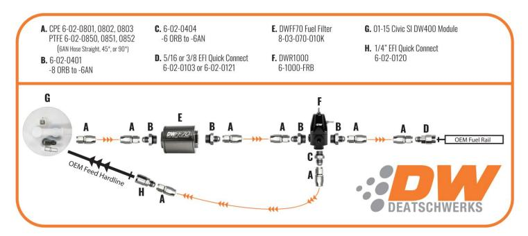
12 – Once you have confirmed the plumbing is correct, you can cycle the key to prime the system, don't start the engine yet, and check for leaks, if leaks are found verify the hose ends are tight, if continuing to leak disassemble and inspect the hose end for proper installation. Once no leaks are present, you can adjust the fuel pressure to the desired pressure, OEM is 50-52psi (3.5BAR). Once the fuel pressure has been set you can start the car. Once running check again for fuel leaks.
