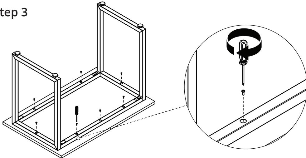
Secure the fixed frame into the desktop using the provided self tapping wood screws
