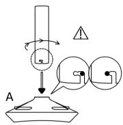
Slide the seat (A) + (B) onto the cylinder (C).
