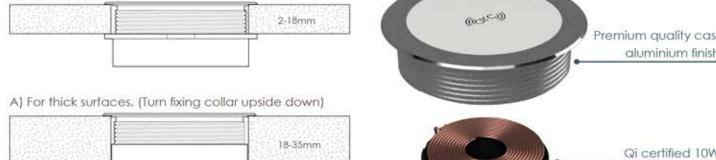
Place ARC-80 into an Ø80mm cutout, and tighten the fixing collar by hand in the position best suited to the thickness of your surface.
