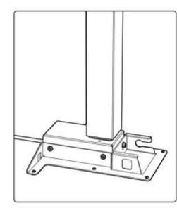
• Insert the 6 screws S-A into the mounting holes and tighten them.
