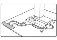
Connect the right cord on the control panel to the motor cord.
