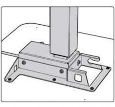
· Align the screw holes on the desktop () with the mounting holes on the support bar. Insert and tighten 6 screws 6-0 from below.
