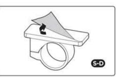
Remove the back film of the under desk cable clip and attach it to the back of the desktop.
