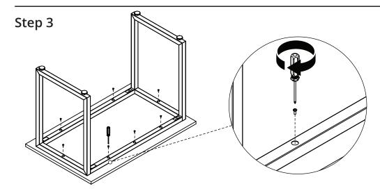
Secure the fixed frame into the desktop using the provided self tapping wood screws
