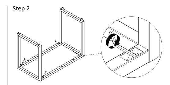
Tighten the 4 large hex screws to secure the legs to the cross bars
