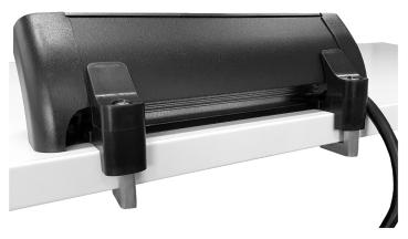
Top fix PACE brackets are positioned at each end and then tightened from the top using an allen key. PACE has easy access at the back to allow for termination of through connectors or pre-terminated data and AV.
