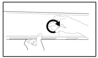
Tighten the centre knob to secture the tray into position. This Will ensure that the component does not move nor slide.
