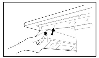
Insert and screw into place the spring loaded release screws into the side bracket (either side).
