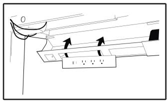
The purpose fit cutouts in the channel fit our powerboards These click seamlessly into the tray.
