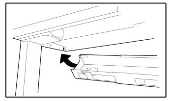
Slide one end of the cable management channel into the side bracket at the back of the Desky.
