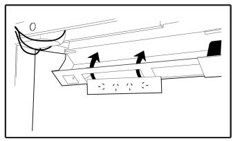
The purpose fit cutouts in the channel fit our Elsafe powerboards - These click seamlessly into the tray.
