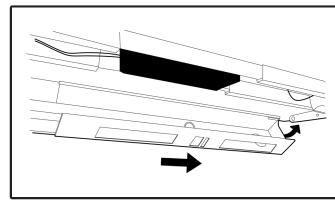
Extend the length of the channel to meet the opposing bracket and secure into place.
