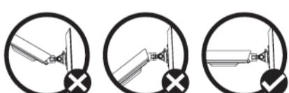
If the arm **drops**, turn the adjustment screw clockwise until it stays in a horizontal position.
