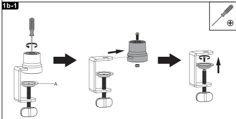
If mounting through desk, remove the clamp using a Phillips head screw-
