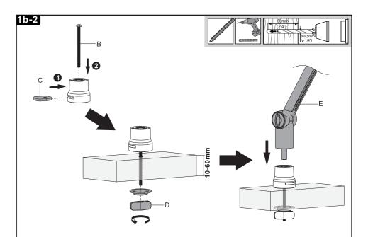
If mounting through the desk drill a hole into your desktop using a 6-8mm drill bit. Insert part C and B into the base (A) and tighten using part D.
