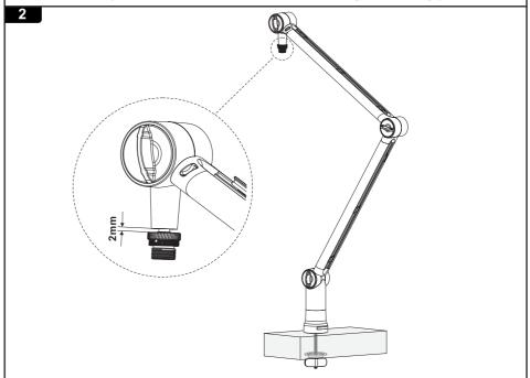
Adjust the boom arm to suit your microphone using the 3/8" or 5/8" screw.
