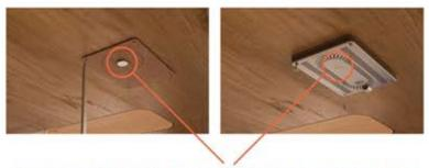
The Magnet and ARC logo indicate the centre of the charging coil. Ensure the module is mounted aligning the desktop decal with the module arc logo
