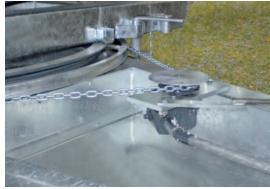
**Option: swivel aid – mechanical or hydraulic** For easy swivelling on uneven grounds
