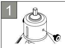
Begin by installing the two thumbscrews in the tool body (near the shank end)
