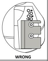
The tenon diameter is variable based on the <u>blade offse</u>t. Smaller offset = smaller tenon, larger offset = larger tenon. Approximate blade offset (in the table above) is a good place to start, but you will want to test tenon fit in holes to achieve the correct offset (we recommend writing the results down). DO NOT set the blades beyond 5/16" or the blade edge will not contact the log and will not cut.
