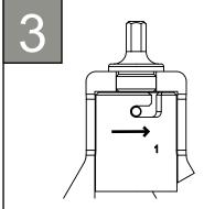
Turn the insert clockwise to lock in place
