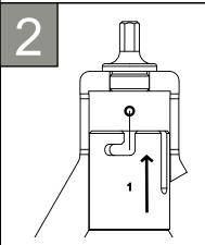
Select the correct size insert based on the desired tenon size
