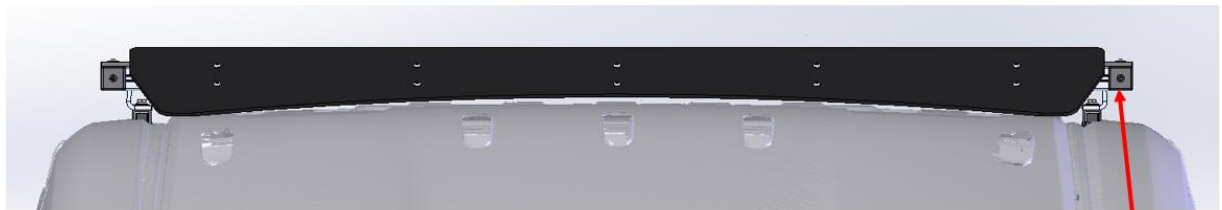
Wind Fairing Installed on 60.25" Cross Bars
