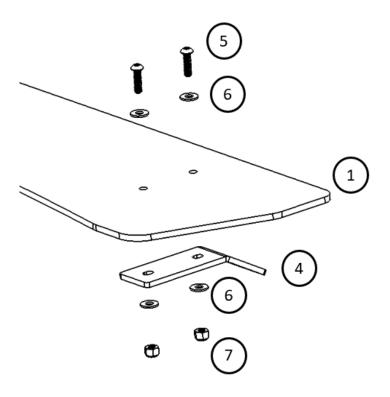
Figure 7: Detailed view showing assembly hardware sequence
