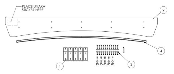
Figure 4: Wind fairing parts provided (Items are not shown to scale)
