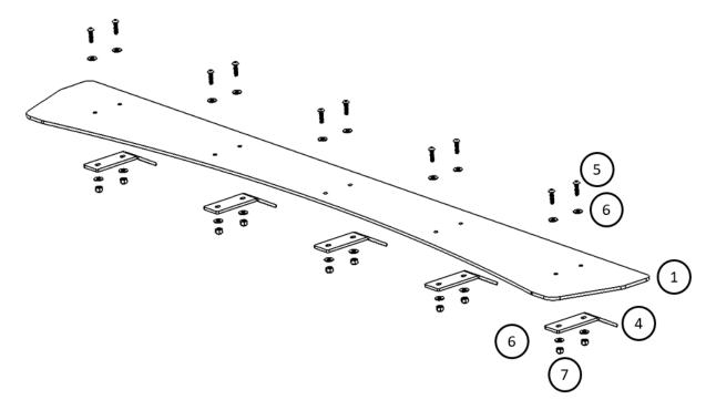
Figure 6: Ram ProMaster Wind Fairing Part Breakdown
