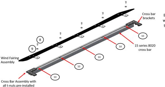
Figure 9: Bolting the wind fairing to an 8020 cross bar
