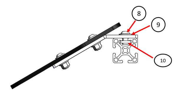
Figure 10: Installation hardware as shown on 8020
