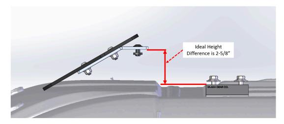
Figure 12: Positioning wind fairing on a custom roof rack
