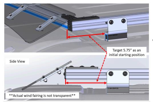
Figure 11: Wind fairing cross bar initial mounting location
