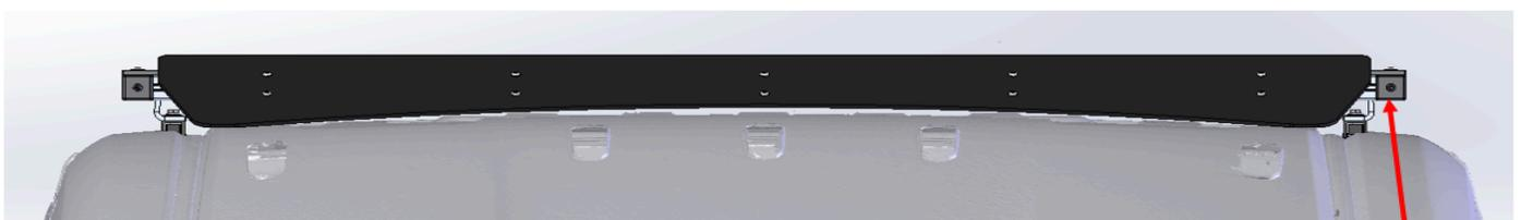
Wind Fairing Installed on 60.25" Cross Bars
