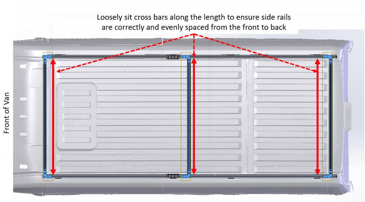
Figure 18: Use cross bars to align side rail assemblies
