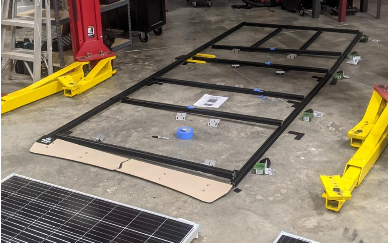
Figure 2: Layout rack on floor including hardware, label parts, hardware quantity, and locations as needed
