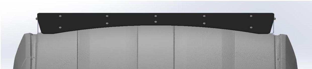
Wind Fairing Installed on 56.125" Cross Bars
