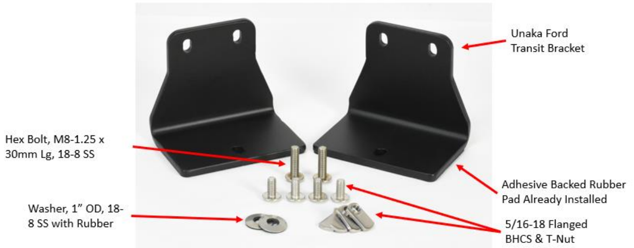
Figure 3: Unaka rack bracket component breakdown
