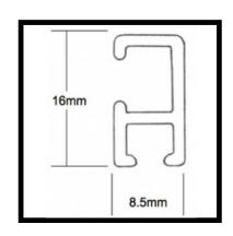
The Australian made Minirail System is currently the smallest picture rail tracking available worldwide, the moulded aluminium profile is just 16.0mm high, 8.5mm thickness and has a load bearing capacity of 25.0 kgs per lineal metre.
