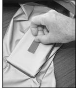
Step 4: Place the patch over the hole, fabric up / smooth film down. Cover the patch and your dry-suit fabric with parchment paper before applying heat. Take your heated iron and apply pressure. Keep the iron moving in a circular motion. In 10 to 20 seconds the film will liquefy. (You will see evidence of this through the parchment paper).
