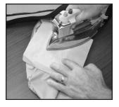
Step 5: Remove the iron and inspect the patch. Take care not to burn your fingers. The adhesive must have melted into the woven fabric "tricot" layer to act as an effective bonding layer. You should see the adhesive oozing out past the edge of the patch.
