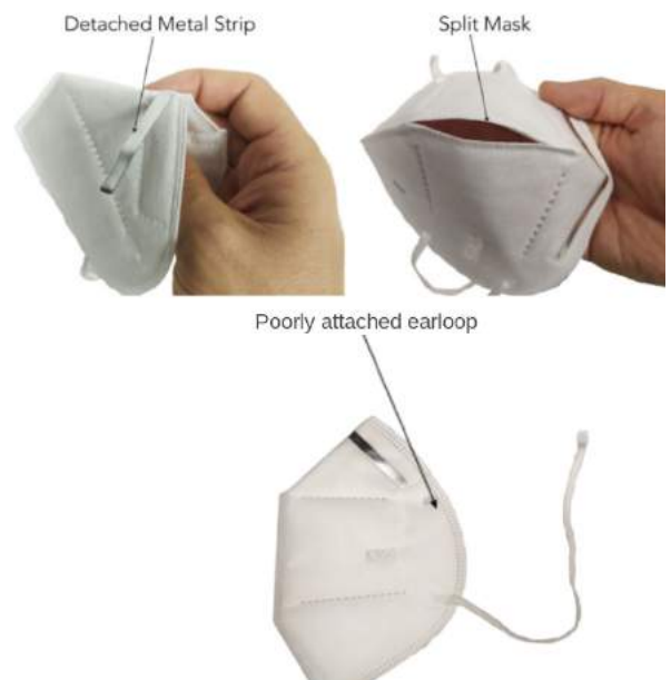
Examples of defects found in some masks sold as KN95s.
