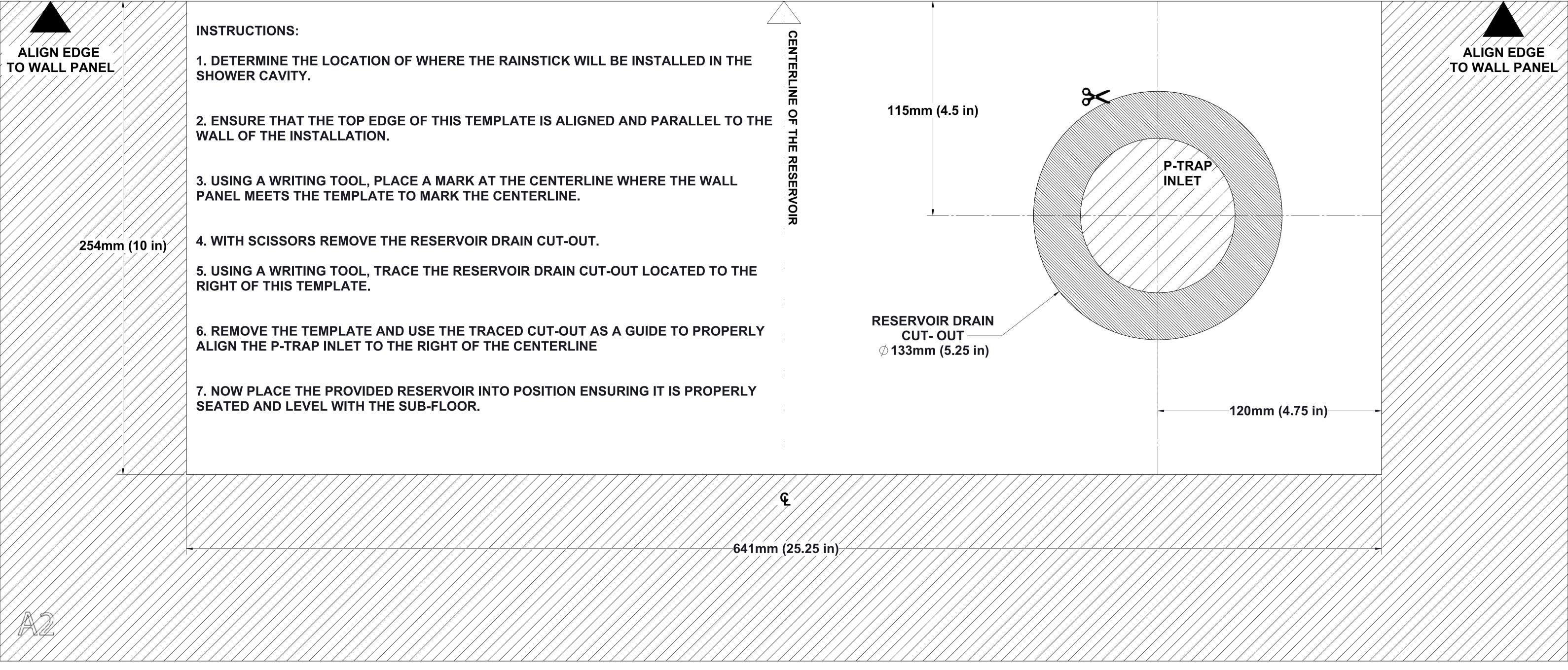
NOTE: HATCHED AREA INDICATES A 101mm (4 in) PERIMETER WHERE INSTALLATION OF A HEATED MAT SHOULD BE AVOIDED.
