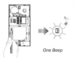
• Press and hold down the programming pushbutton until the Door lock LED starts flashing, and a confirmation sound is heard.
