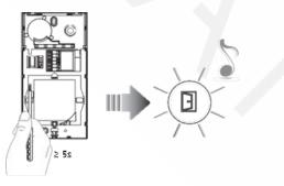
Press and hold down the programming pushbutton until the Doorlock LED starts flashing, and a confirmation sound is heard.
