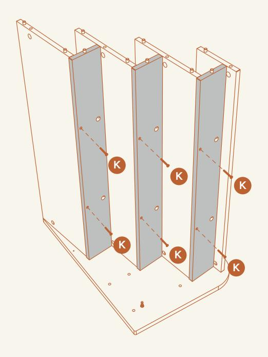
Insert Part C & D panels into Part B. Ensure all the respective parts have been insert into Part B with the holes facing on the correct side as seen below. Lock Part J (1x) turning clockwise until tightened.
