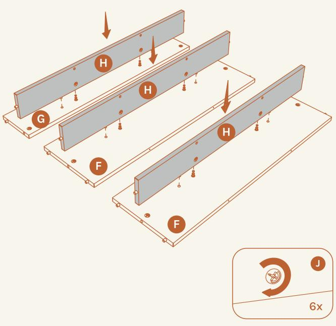
Turn the cam lock nuts (J) clockwise until tightened
