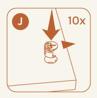
Arrow on cam lock nut to face the edge
