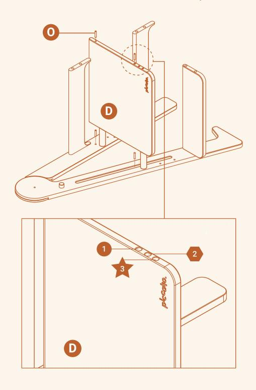
Insert Part D into Part A and B using Part O.
