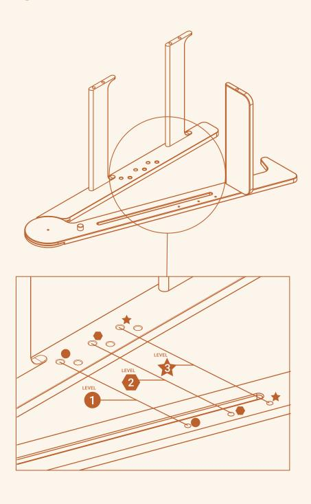
Screw in 2x Part G into legs Part B and Part A.
