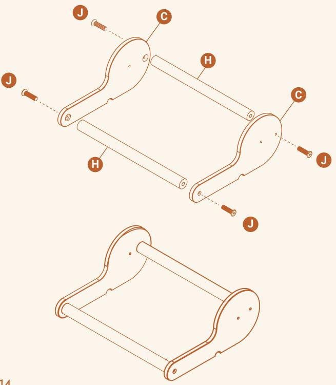
Connect handle from Step 9 to main body on both sides.
