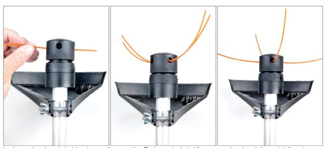
Load your nylons that suit the job and power of your machine. The best option is doubling up your nylons through the one hole for optimum cutting power and efficiency.
