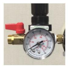
SLOWLY open ball valve let the air pressure slowly build up, as this will prime the pump. (Never take the pressure over 50 PSI.)
