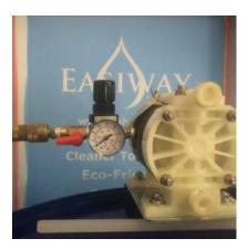
Attach air source to pump regulator. (Note: the gauge and regulator are preset, pump should be run at no more than 40 PSI.)
