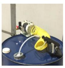
6. To use, pull trigger back to prime pump and apply spray to screen.
