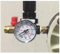
3. Make sure the ball valve on air inlet is closed and attach the air line.
