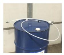
1. Place 3/8" line through the 3/4" drop tube and replace the coupler on the end of the 3/8" line, and attach to pump.
