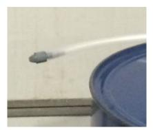
Place the drop tube/line into drum (pulling foot valve tight against tube) gently thread bung cap into place.
