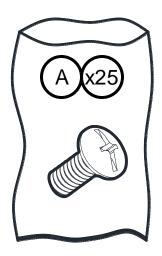
Truss head screw 5/32-32 x 25/64"
