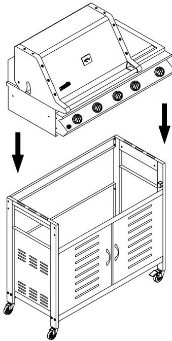
STEP 10: Secure the head unit to cart use 4-truss head screws (1/4" x 15mm) with lock washers and flat washers as shown on diagram below. (Note: Remove cooking grids and flame tamers before this step)
