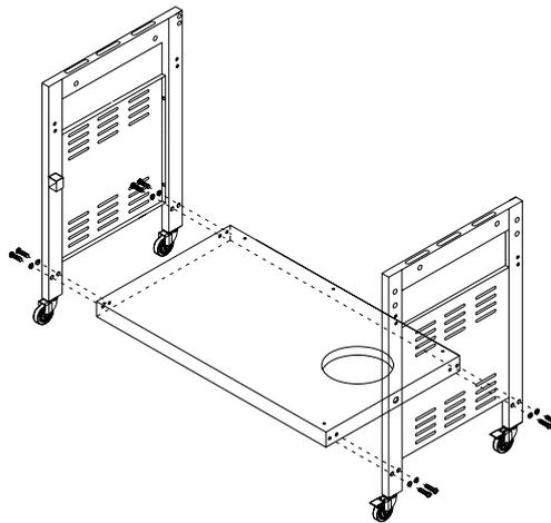
STEP 3: Assemble back panel to side panel legs with 6 (5/32" x 8mm) truss head screws as shown figure below.
