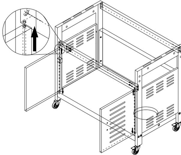
STEP 6: Attach center door flame with bottom panel and front flame use 4 pieces (5/32"x10) screws.
