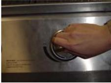
Step 2. Press the electric igniter 3 to 4 seconds to light the rotisserie burner
