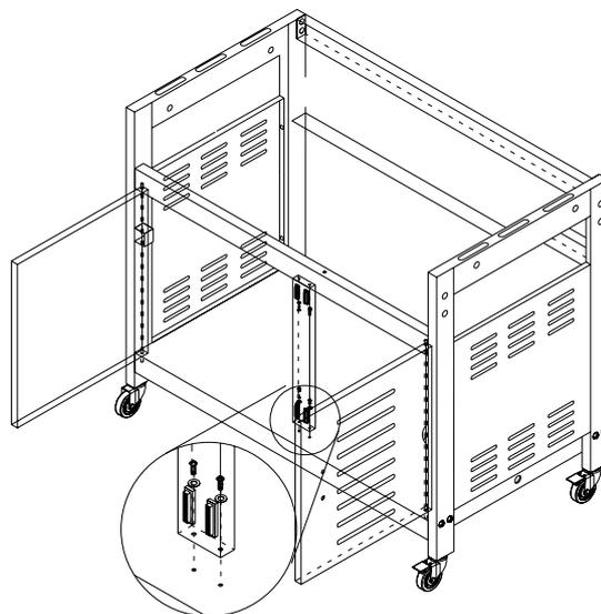
STEP 7: Assembly barrier shelf to the left side panel leg, back panel and center door frame with bottom panel and front flame use 4 pieces (5/32"x10) screws.
