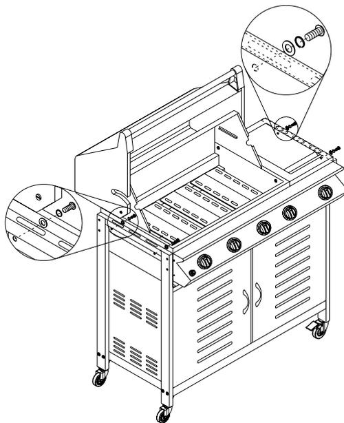
STEP 11: First secure the push bar to the right side shelf use 2 pieces truss head screws (1/4" x 15mm) with flat washers and lock washers second attach the side
