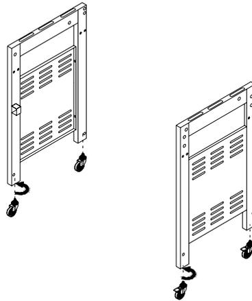
STEP 2: Attach bottom panel to side panel legs use 8 pieces truss head screws (1/4" x 40 mm) with 8 pieces 1/4" lock washers and flat washers to secure bottom panel and side panel legs.
