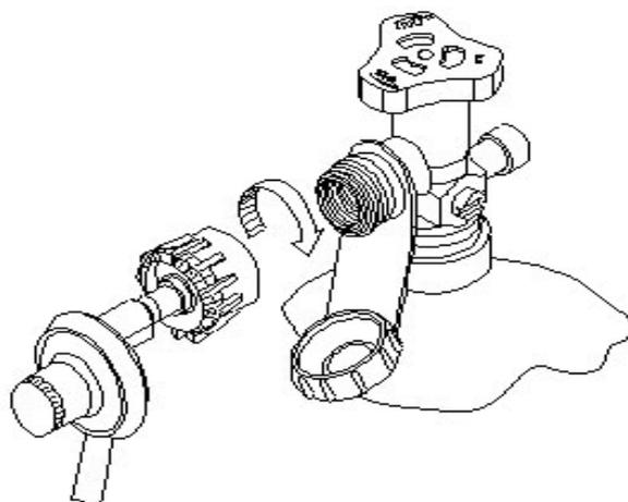
*NEVER CONNECT AN UNREGULATED GAS SUPPLY LINE TO THE APPLIANCE. USE THE REGULATOR/HOSE ASSEMBLY SUPPLIED.*
