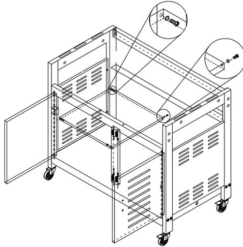
STEP 8: Assembly door handle to the door with 4 pieces (5/32"x10) screws on the each side.
