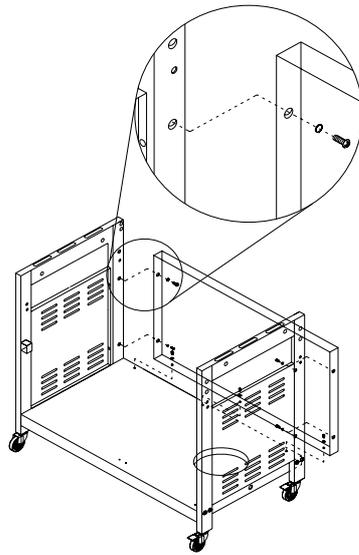
STEP 4: Fix cart frame cross bar to both side panel-legs with 4 (1/4" x 15mm) truss head screws with lock washers and flat washers.
