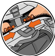
Open the zip fastening on the airbag compartment completely so that the zip is only running on one side of the fastening. Push the zip all the way up and reconnect the ends of the fastening.
