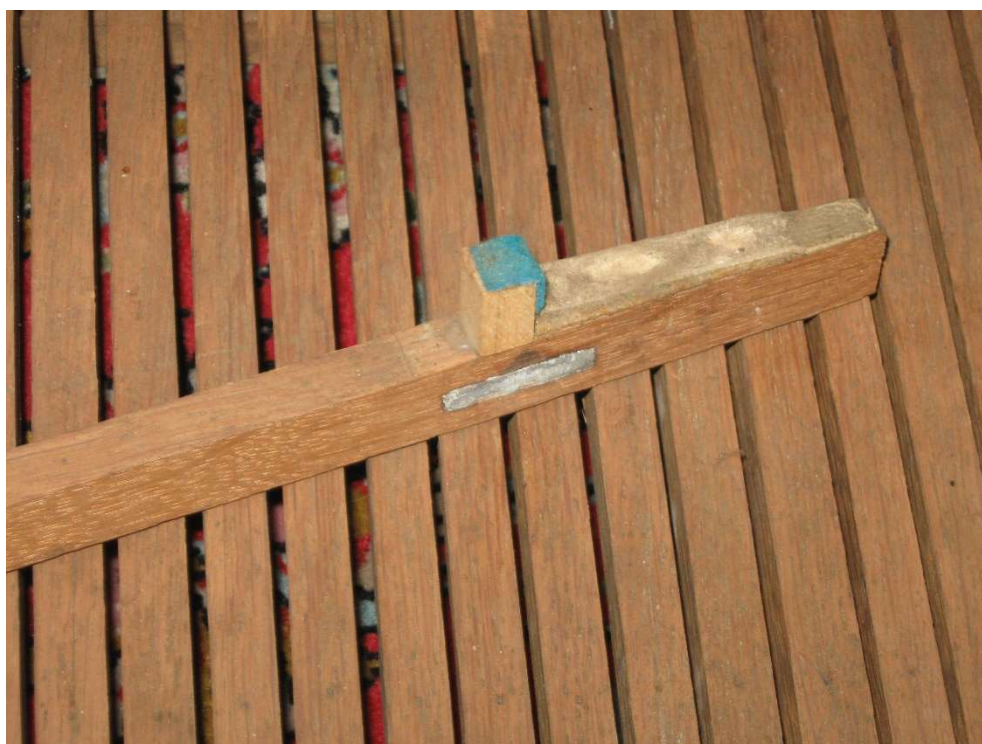
A lower-manual key lever with added coupler block
