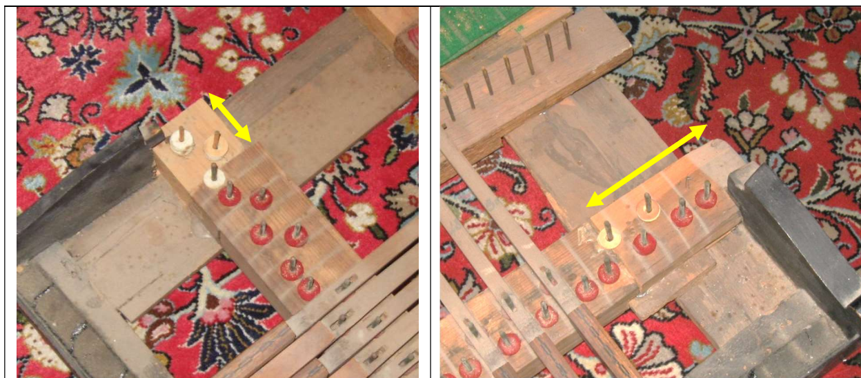
Figure 37. The arrows indicate the additions to the bass and treble ends of the balance rail.
