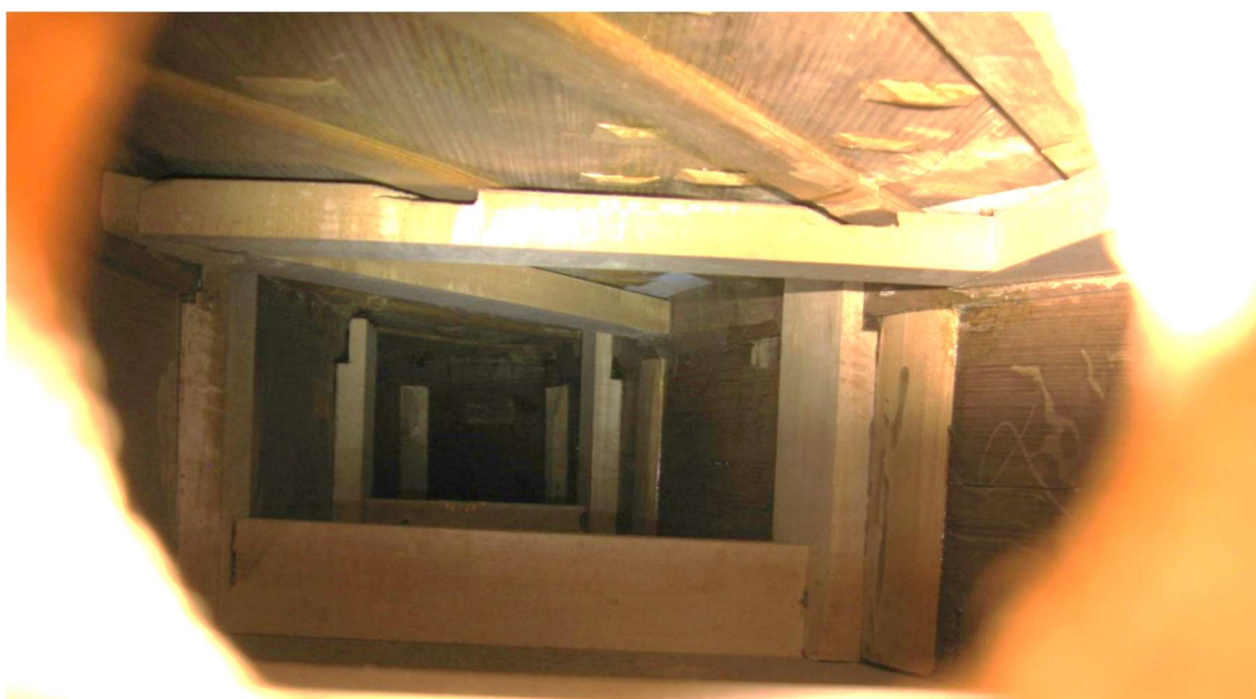
Figure 18. The interior under the soundboard, viewed through one of the holes in the belly rail.
