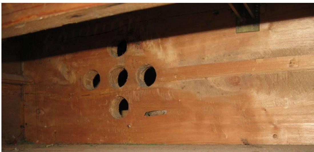
Figure 17. The modern belly rail with its set of holes in the bass; another set is in the treble.
