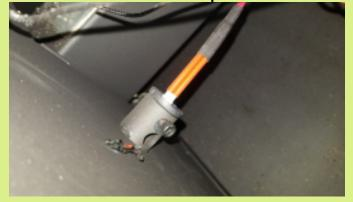
Loosen the clamp screw using a #5 Metric Allen wrench to make adjustments
