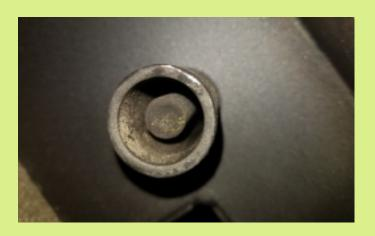
If adjustment is required, locate the set screw that holds the igniter rod clamps in place. These are accessible through the removable side panels
