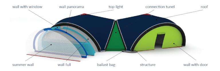
Structures consist of bladder made of TPU and fabric part made of Duratex FR fabric.
