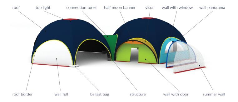
Structures and tubular parts of visors consist of bladder made of TPU and fabric part made of Duratex FR fabric.
